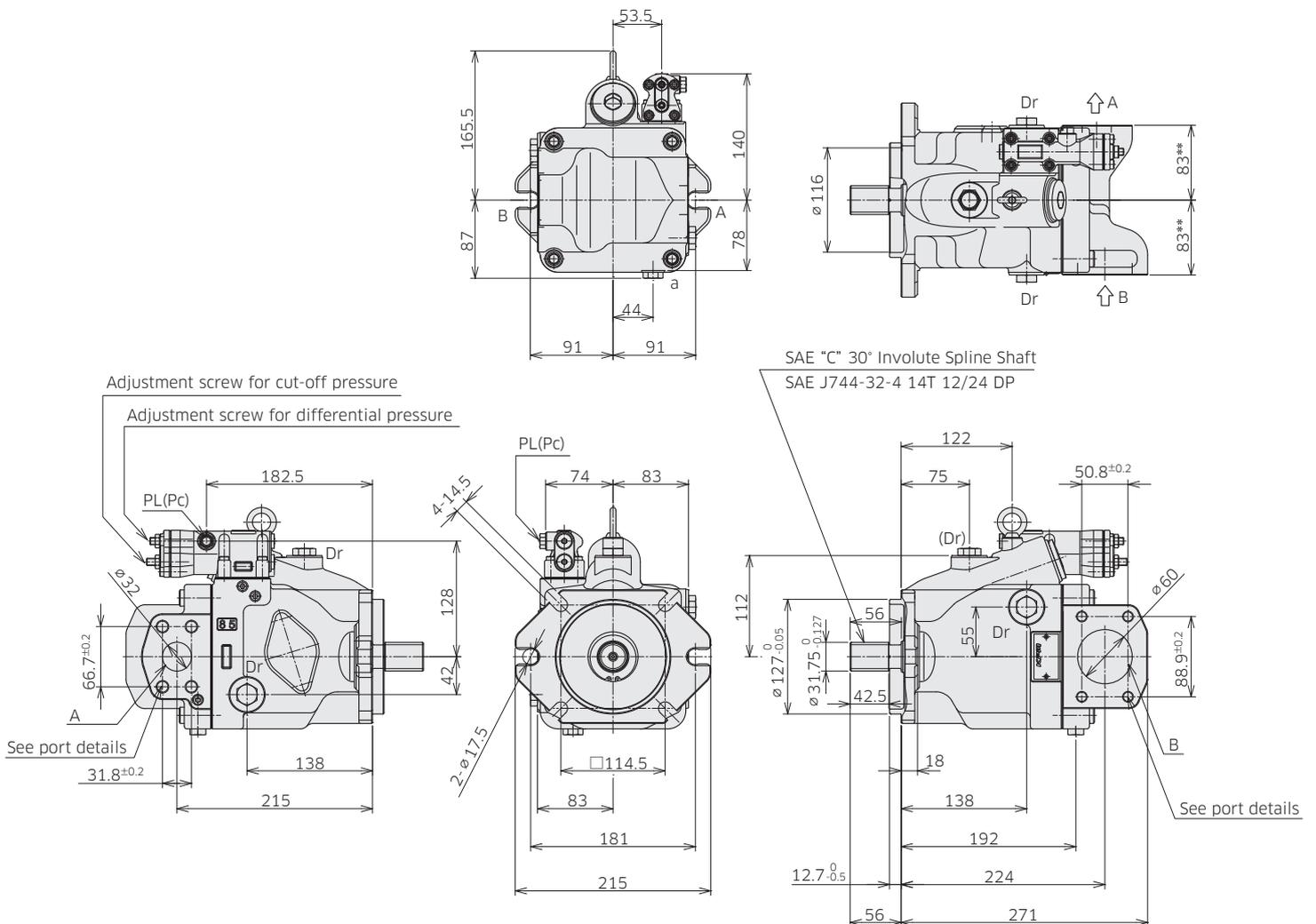
Involute spline according to ANSI B92.1a, 30° pressure angle, flat root, side fit.
