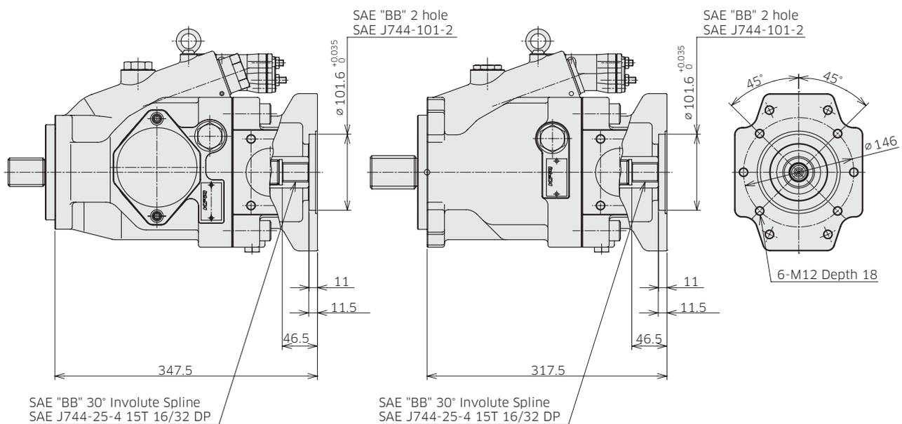
Involute spline according to ANSI B92.1a, 30° pressure angle, flat root, side fit.
