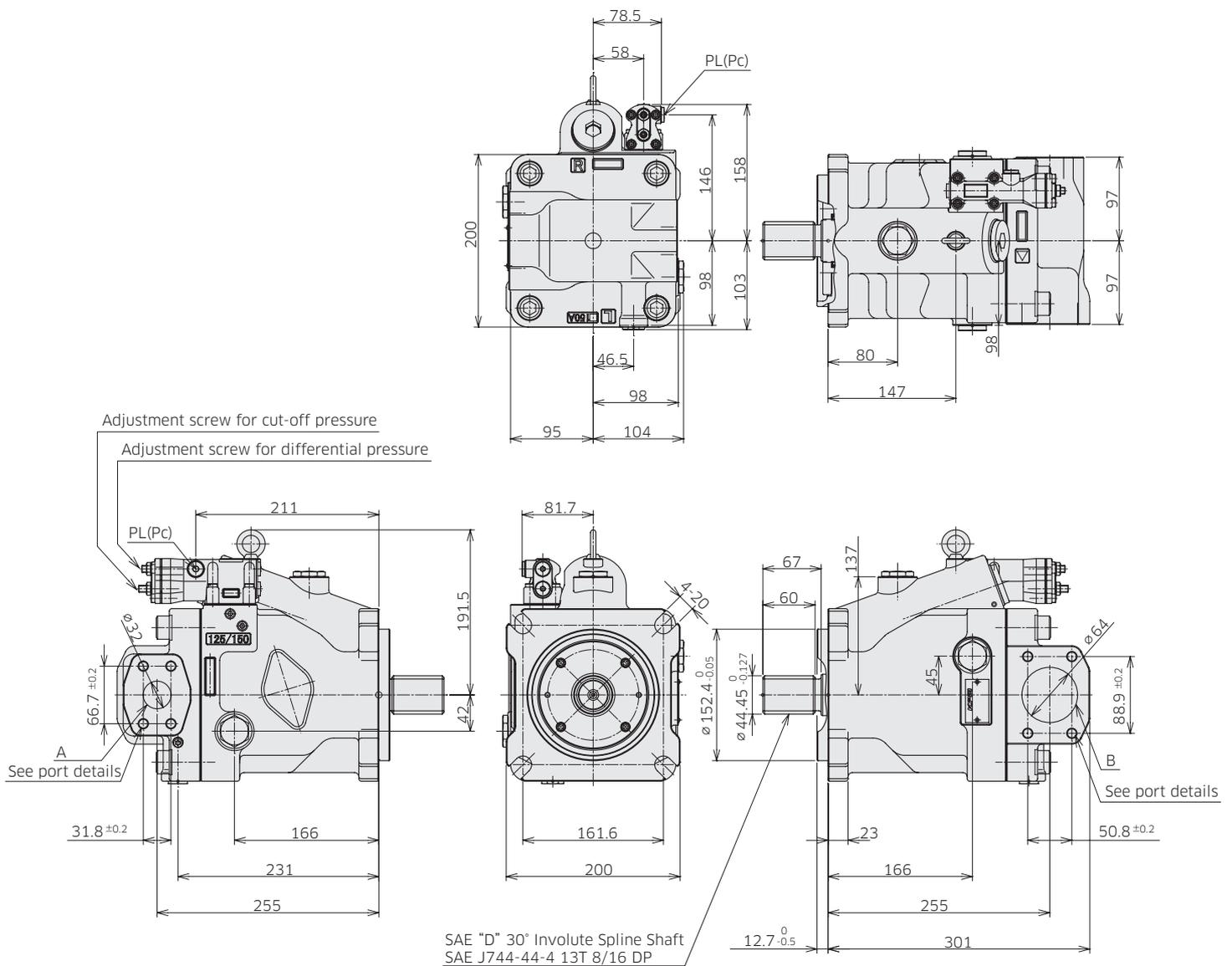
Involute spline according to ANSI B92.1a, 30° pressure angle, flat root, side fit.
