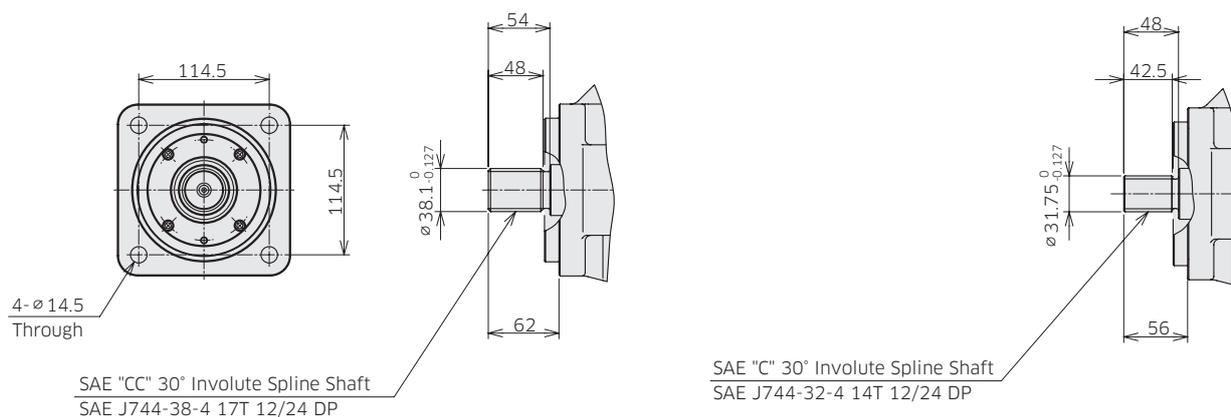
Involute spline according to ANSI B92.1a, 30° pressure angle, flat root, side fit.
