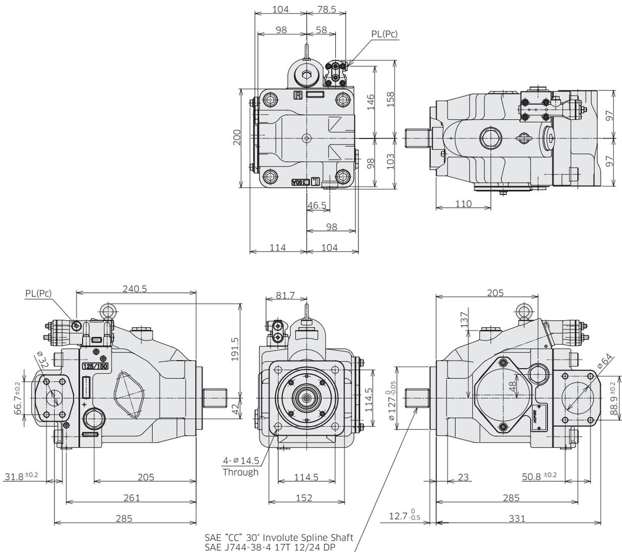
Involute spline according to ANSI B92.1a, 30° pressure angle, flat root, side fit.
