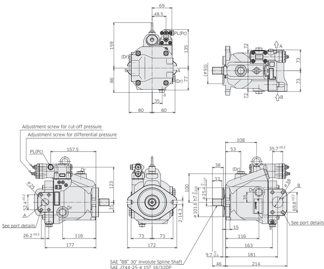
Involute spline according to ANSI B92.1a, 30° pressure angle, flat root, side fit.
