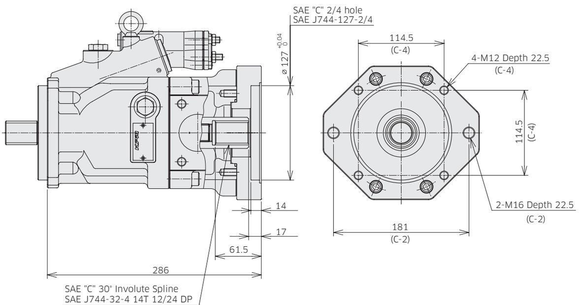
Involute spline according to ANSI B92.1a, 30° pressure angle, flat root, side fit.
