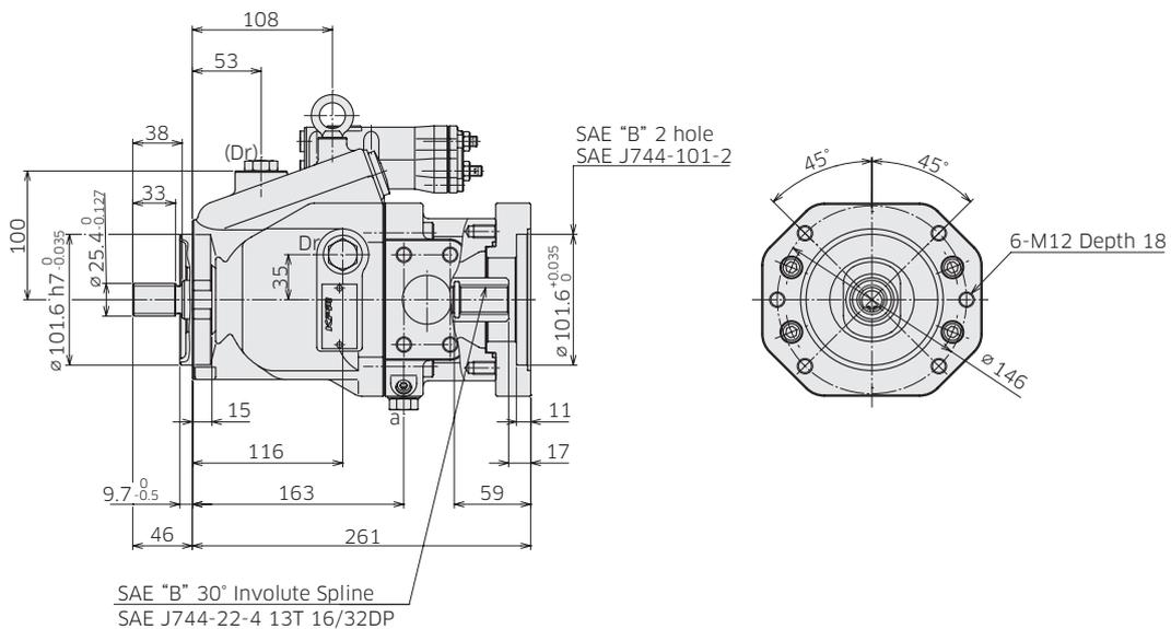
Involute spline according to ANSI B92.1a, 30° pressure angle, flat root, side fit.
