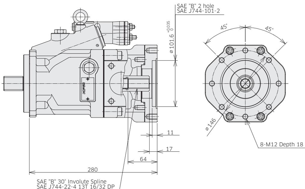
Involute spline according to ANSI B92.1a, 30° pressure angle, flat root, side fit.
